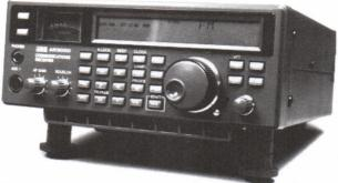
Six bandwidths are supplied (3, 6, 15, 40, 110 and 220 kHz.) and a slot for a .5 kHz filter is available. The triple conversion circuit and varactor tuned front-end provides excellent overload characteristics. One thousand memories in 10 banks of 100 are featured. Other features include: two antenna inputs, antenna attenuator, keypad entry, computer control, squelch, S-meter and scanning. May be run from 12 VDC (1 Amp) or via supplied AC adapter.
