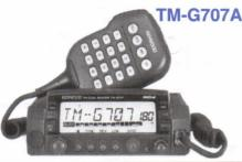
From the extra-large control panel — with the welcoming glow of its amber-colored LCD - to Kenwood's new Easy Operation mode, the TM-G707A is extraordinarily user-friendly ... an important consideration for a mobile rig. The TM-G707A offers features such as: memory name function, S-meter squelch, time-out timer, encode/decode, dimmer, auto power-off and supplied MC-53DM backlit DTMF mic. Non-simultaneous cross-band repeater access is supported.
