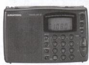
The Traveller III Digital is small on size, but big on features. Coverage includes AM, FM and SW from 2.3-7.4 and 9.4-26.1 MHz. Tuning is via Up/ Down buttons, auto search, direct keypad entry or via 20 memories. A digital quartz clock, with sleep timer, wakes you to a beep or radio. Also has lock button, 9/10 kHz MW step and stereo/mono switch. With carry case, stereo earbuds and Grundig SW Guide. Requires three AA cells (not supplied) or 4.5 VDC. 5.5"W x 3.5"H x 1.3"D. \$89.98 (+\$6)
