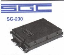
The SG-230 Smartuner™ is a microprocessor controlled automatic antenna tuner operating in the range of 1.6 to 30 MHz with 3 to 150 watts of input power. It has a 500 address nonvolatile memory and tunes antennas from 8 to 80 feet. In compact weatherproof case. 12"x16"x3" \$479.95 (+\$9) SG-230 Order #2834
