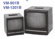
The ProVideo VM-901B monitor is just right for those requiring a high-quality, small metal cased composite monitor. This 9 inch diagonal video monitor provides > 800 lines resolution. Front controls include: Power, Contrast, Brightness, Horizontal Hold and Vertical Hold. Rear composite input .5-2V p-p sync. neg. with BNC jack. Input impedance is High or 75 Ohm switchable. Black metal case 8.6"W x 9.5"H x 10"D 13 Lbs. 120 VAC 60 Hz. (Not for use with M-8000).
