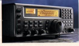
IC-R8500 The expert's choice. 0.5 – 2000 MHz\*; commercial grade; all mode; IF shift; noise blanker; audio peak filter (APF); 1000 memory channels; built-in CI-V command control and RS-232C port for easy PC remote control with ICOM software for Windows®.
