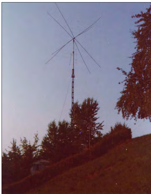
Dreiband 1\frac{1}{2} Lambda-Quad: 20m, 15m, 10m
